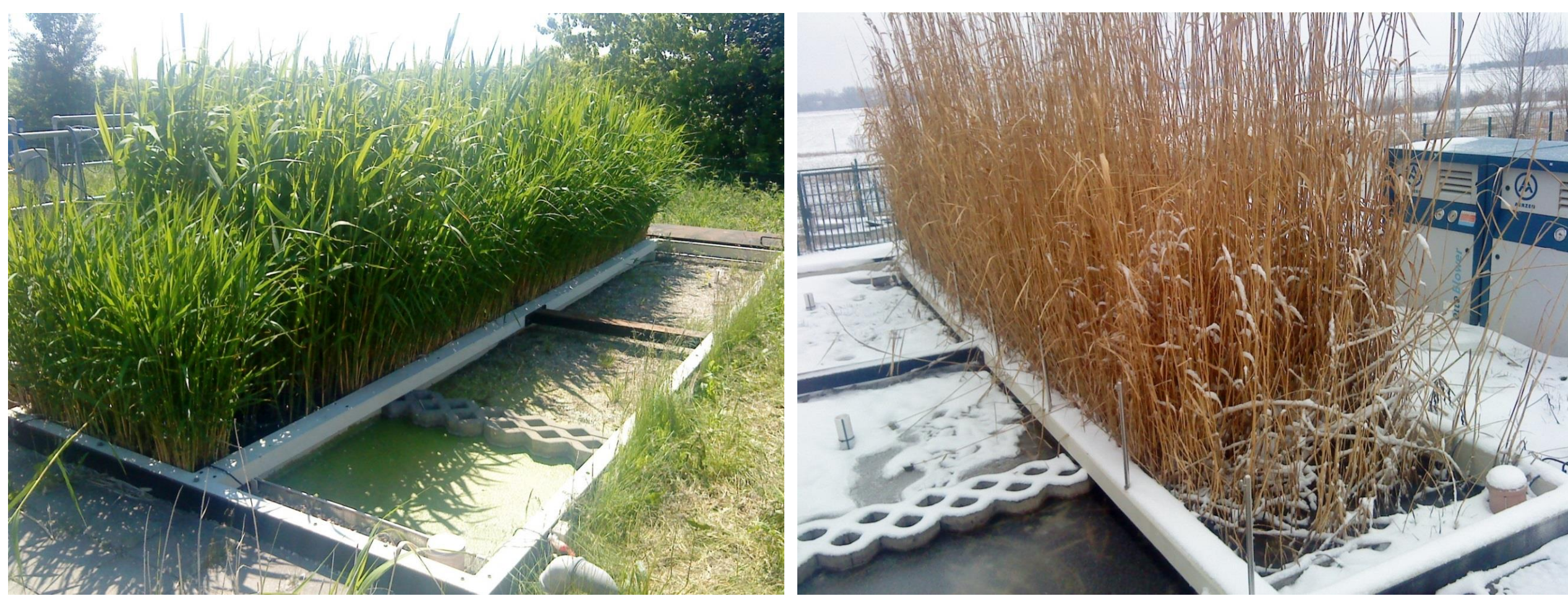
Fig. 2. Pilot CWs (planted/unplanted) during summer and winter operation
