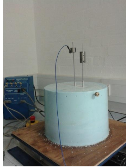
Figure 9 Test models realized in the laboratory and placed over a shaking table for a) single structure and b) structure coupled with ViBa.
