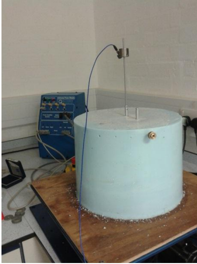
Figure 9 Test models realized in the laboratory and placed over a shaking table for a) single structure and b) structure coupled with ViBa.
