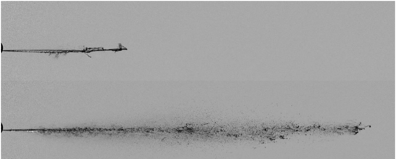
Figure 5. Spray evolution of a low viscosity oil
