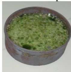
Fig 5. Smooth surface of TinGlass unit produced by melting glass cullet
