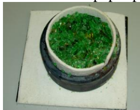
Fig.9 Glass cullet in round steel mould is prepared for the furnace
