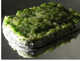
Fig. 6. Rectangular non-smooth glass brick produced by fusing in a sardines' can mould (Photo taken by Mr H. Hills, SET, UoB)
