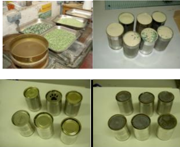
Fig.6. Stages of RG's 1 st sieved granulated glass, 2 nd after placed the tin can, 3 rd after placed the lid, 4 th after placed the appropriate weight on the top of the lid before put in the oven.
