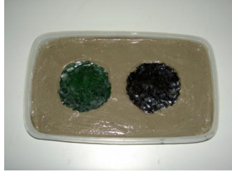
Fig1a. Fragment of wall finish with TinGlass units. This is seen as a take on the traditional flint wall technique as shown in Fig 1b.
