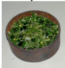
Fig. 4 Non-smooth surface of TinGlass unit produced by fusing glass cullet
