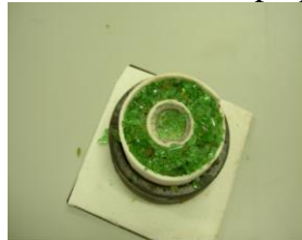
Fig.10 Hollow mould with glass cullet is prepared for placing in the furnace
