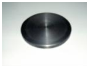
Fig. 5. Cylindrical dick of 150gr of weight and diameter 67mm t placed on the top of the lid
