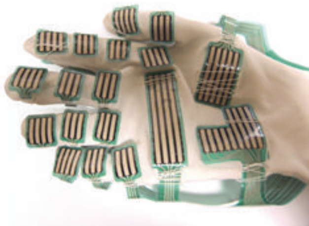
FIGURE 6: The preinstrumented glove showing the Grip attached to the vinyl glove [27]. Photographs courtesy of SATRA Technology Centre.
