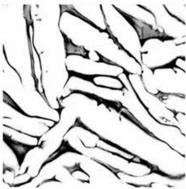
Mean pore size 76 \mu\text{m}
