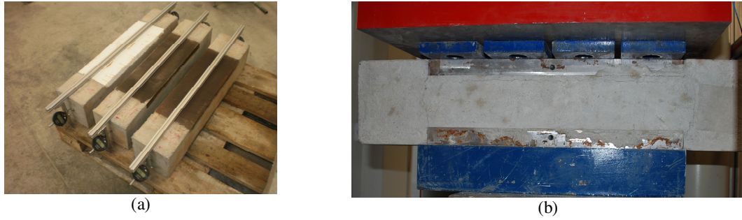
Figure 2: Experimental setup a) for the measurement of shrinkage strain and b) for the compressive testing.
