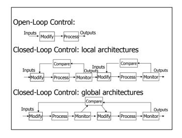
Improvements in the performance and capacity utilisation of a system are made possible by innovations that improve the accuracy, speed, scope and reliability of the control system.
