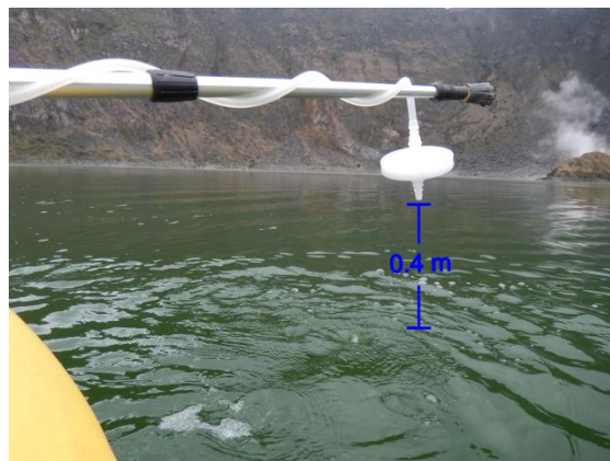
Figure 2.7 – Measurement method with the Multi-GAS at El Chichón (Mexico)
