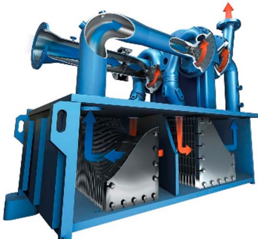
Figure 1. Integrally Geared Air Compressor Cutout
