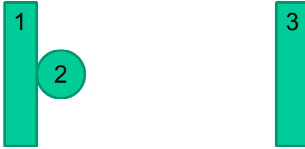
Figure 15 Schematic for modeling the capacitance of the sphere between two planar electrodes
