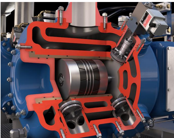
Figure 1: Piston with rings and riders in a cylinder of a reciprocating compressor
