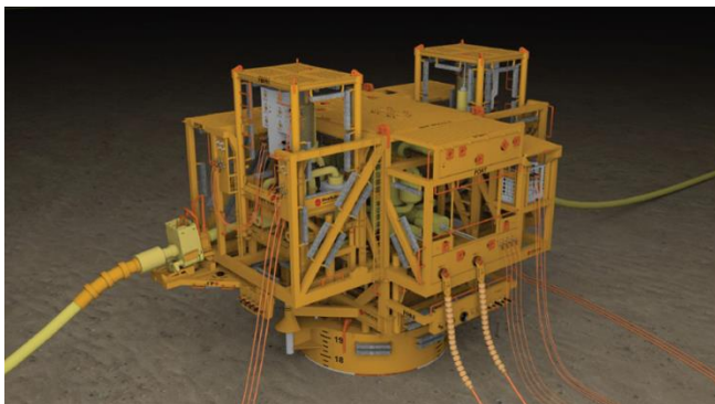
Figure 1 View of the HighBoost MPP station
