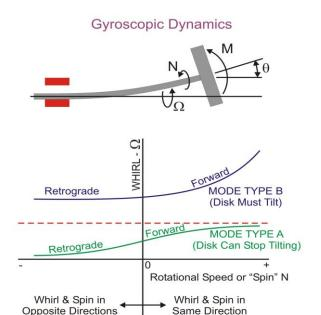
Figure 8. Illustration of Gyroscopics: Effect of Speed (Spin) on Critical Speeds (Whirl)
