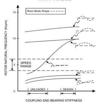
Figure 17. Variation of Rotor Critical Speeds with IB Bearing Stiffness
