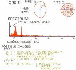
Figure 9. Subsynchronous Vibration
