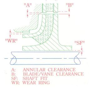
Figure 13. Various Impeller Gaps of Importance
