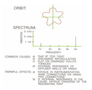
Figure 12. Vane Pass Vibration
