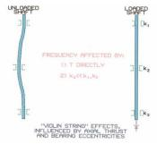
Figure 16. Vertical Pump Lineshaft Rotor Behavior
