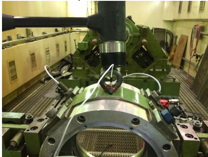
Figure 17: DH4 Vertical Impact Location and Accelerometer Placement
