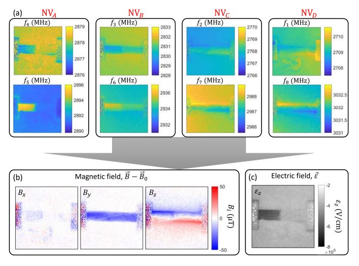
FIG. S10. (a) Maps of the frequencies  $\{f_i\}_{i=1..8}$  obtained by fitting the ODMR spectrum at each pixel. The region shown is the same as that in Fig. S8a, and the bias magnetic field is  $\vec{B}_0 \approx (35, 13, -50)$  G. (b,c) Maps of the magnetic field components (b) and out-of-plane electric field component  $\mathcal{E}_z$  (c) obtained after reconstruction. In (b) a plane subtraction was applied to remove the background field  $\vec{B}_0$ .
