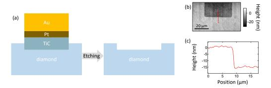
FIG. S13. (a) Illustration of the etching process: the TiC layer formed by annealing is etched away, leaving a recess. (b) Atomic force microscopy (AFM) image of a region thus etched. (c) Line cut extracted from (b) revealing a  $\approx 15$  nm etching step.
