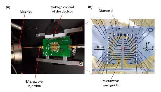
FIG. S5. (a) Photograph showing the PCB with microwave and DC inputs, as well as the permanent magnet used to apply the bias magnetic field  $\vec{B}_0$ . (b) Photograph of the diamond as mounted. The red box indicates a typical area used for imaging.
