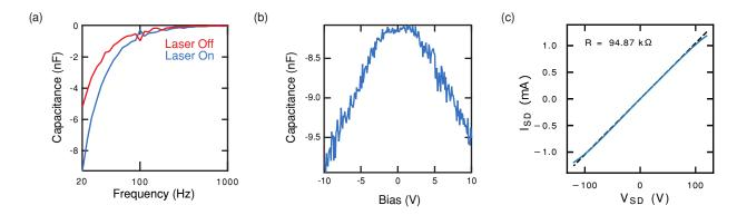
FIG. S11. Electrical characterisation of a representative H-terminated channel between two TiC/Pt/Au contacts. (a) Capacitance under a bias voltage  $V_{DS}=10$  V, as a function of the frequency of the AC signal. (b) Capacitance at 20 Hz as a function of the bias voltage (laser on). (c) Source-drain current as a function of the applied DC voltage.
