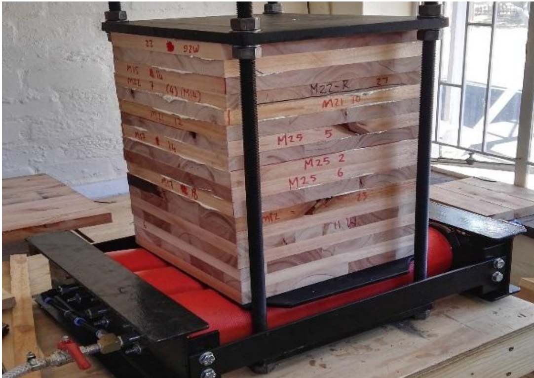
Figure 3-8: CLT press loaded with six CLT panels under pressure.
