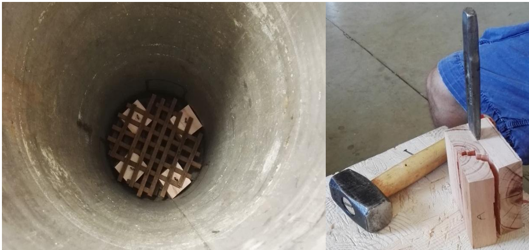
Figure 3-12: Samples in autoclave, weighed down and about to be submerged in water (left) and hammer and chisel used to split the glue line to estimate WFP (right).
