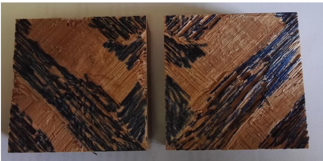
Figure 3-16: WFP (approximately 60%) of a 70 x 70 sample. Blue indicates wood failure.
