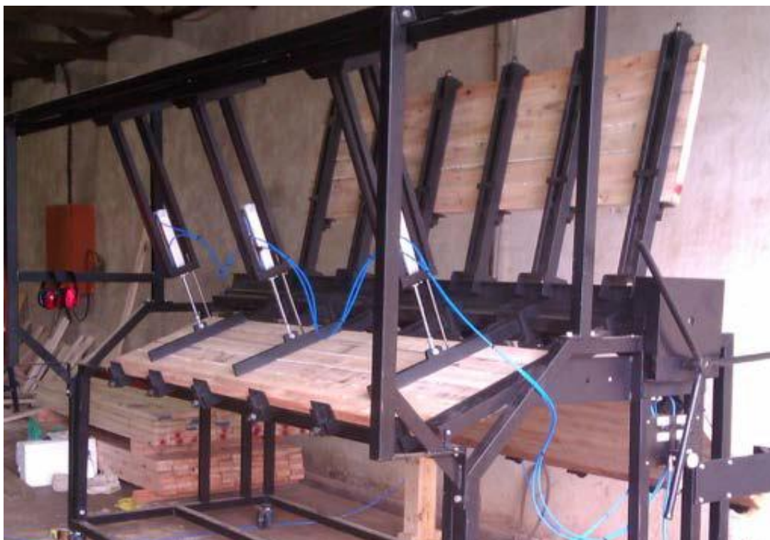
Figure 3-4: Edge laminating press fully loaded with 3 panels. Vertical clamps are applying pneumatic pressure to flatten the panel, while six clamps are applying 0.75 MPa of pressure for edge bonding.
