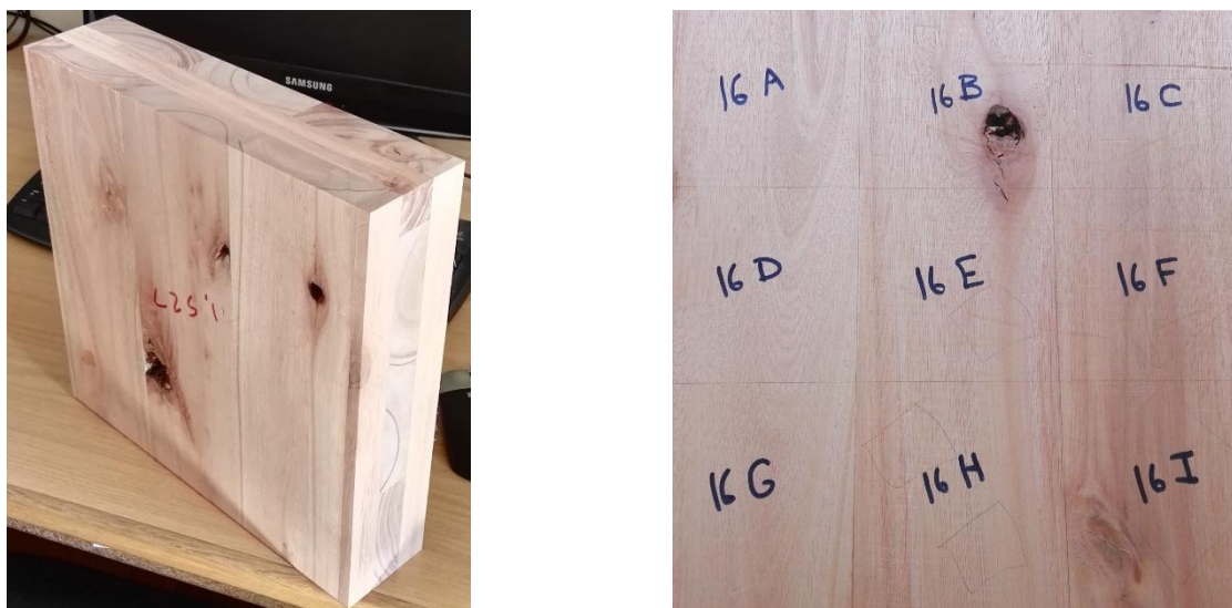
Figure 3-9: Finished CLT panel (300 x 300 x 75 mm) (left) and panel 16 of 40 with the positions marked (A – I) (right)
