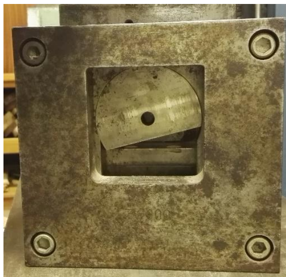
Figure 3-13: 40 x 40 sample showing shear test method (left) and shearing tool with self-aligning cylindrical bearing (right).
