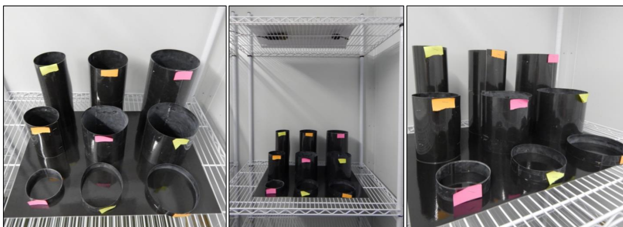
Figure 4: The experimental setup of the flight cylinder matrix assessment, with matrix of nine flight cylinders using all combinations of cylinder heights (2.5, 15, and 26.5 cm) and diameters (10, 14 and 16 cm). The cylinder placement was randomized during experiments, with the coloured pieces of paper indicating the treatment that was placed in the specific cylinder.
