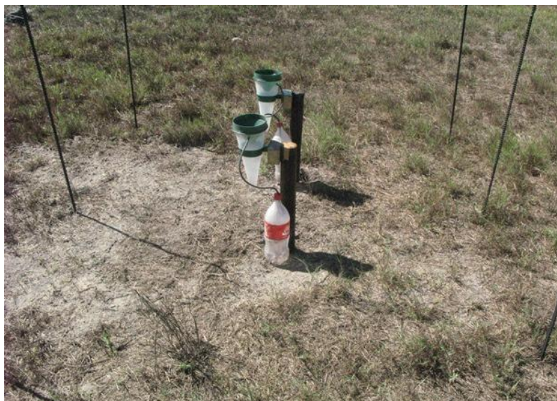
Figure 3.3. Rain gauge with attachment to catch overflow for measuring the volume of wastewater applied to a replication plot at a winery near Stellenbosch.
