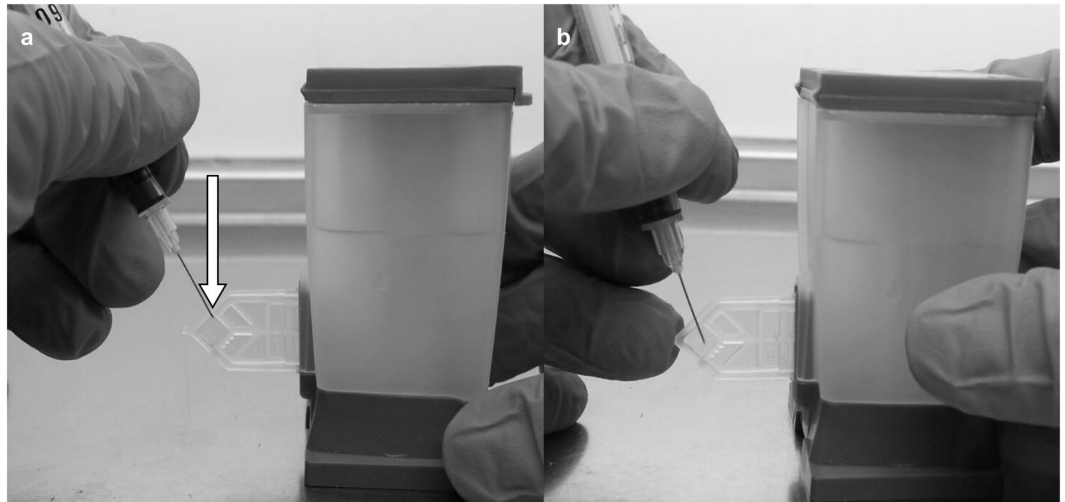
Figure 1. Cartridge extract extraction procedure. (a) The arrow indicates the diamond-shaped reaction chamber where the PCR amplification takes place and contains cartridge extract with mycobacterial genomic DNA. The needle is placed at the top of the diamond and the film is slowly and carefully pierced. (b) The needle is then slowly inserted deeper into the pocket and cartridge extract mix drawn out without piercing the other side.
