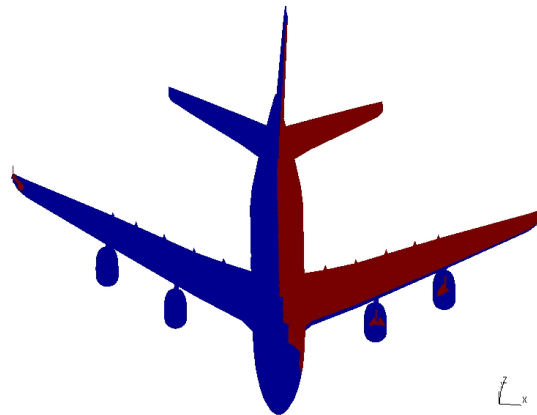
Fig. 7. Shadowing judgment result for electric dipole illumination. Red = illuminated; blue = shadowed.
