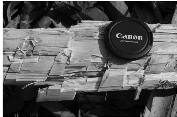
Figure 1: Log surface damage in smaller diameter logs inflicted by harvester head feed rollers and delimiting knives.
