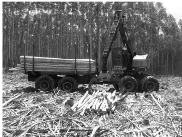
Figure 8: Primary transport of logs by forwarder.
