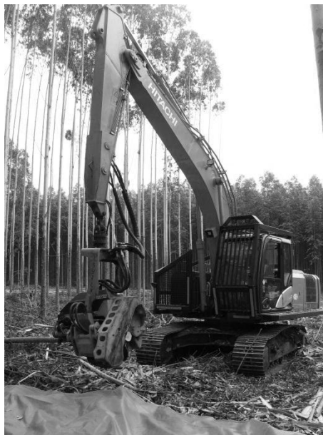
Figure 5: SP Maskiner 591LX harvesting head mounted on a tracked Hitachi IS200 excavator.
