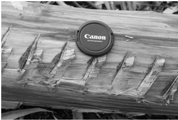
Figure 1: Log surface damage inflicted by harvester head feed rollers and delimiting knives.
