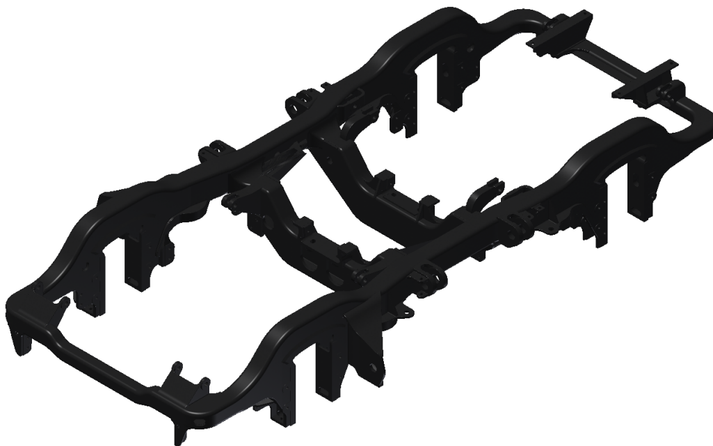
Figure 5.2: Three dimensional model of 5M bogie frame
