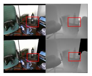
Figure 7.40: This demonstrates the Kinect's inability to handle very reflective surfaces as seen in this image. This image shows four views of the surface, the top left image is the raw RGB image, the top right image illustrates the bilaterally filtered depth image and the bottom images show the view from the RGB volume and the TSDF volume. A reflection of the surface behind the box is shown on the box. The IR light is being reflected.
