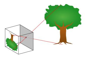
Figure 2.1: The basic pinhole camera model illustrates the reflected light from a tree entering the box through the aperture and falling on the interior surface at the rear of the box.
