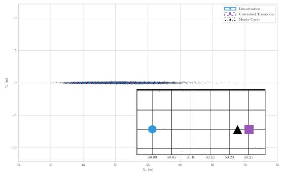
Figure 3.6:  $X_r - Y_r$  projection of 3D feature distribution for a distance of 50.0 m from the stereo camera pair. Subplot indicates magnified area around approximated means.
