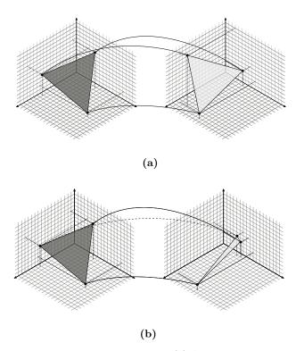
**Figure 6.5:** Illustration of PORUS for visual odometry. (a) A triple of three dimensional points, without outliers, undergoing a rigid body transformation. The triangle formed is invariant across viewpoints. (b) The same triple of points undergoing a rigid body transformation where an outlier is introduced in the second viewpoint (dashed line). A clear change in shape is observed.
