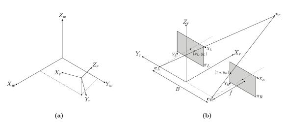
Figure 5.1: Simulated robot coordinate frames. (a) Illustration of robot state vector in world coordinate frame. Thirteen robot states are described by the robot's position vector and orientation quaternion,  $\mathbf{r}_w$  and  $\mathbf{q}_w$ , as well as the linear angular velocities,  $\mathbf{v}_w$  and  $\boldsymbol{\omega}_w$ . (b) A rectified stereo camera pair centered on the robot frame.
