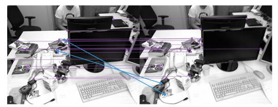
Figure 1.3: Illustration of outliers (mismatched features). Outliers, depicted by blue circle markers, are introduced during feature matching and are inconsistent with the camera motion between viewpoints. Image frames are part of the  $TUM RGB-D Benchmark^4$  [70].
