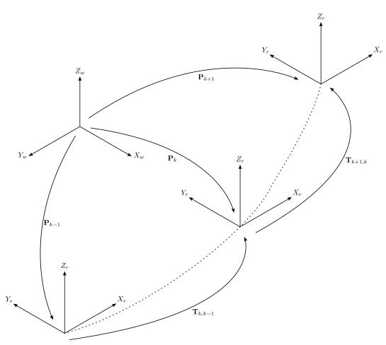
Figure 1.2: Graphical representation of the visual odometry problem for a robot moving along an abritary path (dashed line). The relative pose (rigid body transformations) between successive time steps,  $\mathbf{T}_{k,k-1}$ , is determined by tracking visual features across viewpoints. Transformations are accumulated over time to obtain the pose of the robot,  $\mathbf{P}_k$ , in the world coordinate system. Adapted from *Visual Odometry: Tutorial* by Scaramuzza and Fraundorfer [36].
