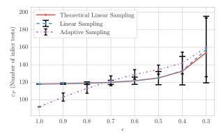
Figure 6.14: Comparison of sampling strategy costs as a function of  $\epsilon$  where the true value of  $\epsilon$  is not observed and an initial estimate of the inlier ratio,  $\hat{\epsilon} = 0.8$ , is used.
