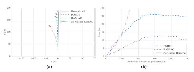
Figure 7.15: KITTI 2009\_09\_08\_drive\_0021 (a) Reconstructed trajectories. (b) Euclidean distance error of estimated trajectories as a function of the number of pose estimates.
