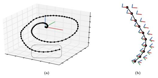
Figure 5.2: An example robot trajectory generated using an acceleration based model. (a) 3D view of the trajectory. (b) A section of the trajectory which has been magnified to illustrate the poses of a stereo pair mounted to the robot. The colours of the axes, R - G - B, correspond to the  $X_c - Y_c - Z_c$  of each camera.
