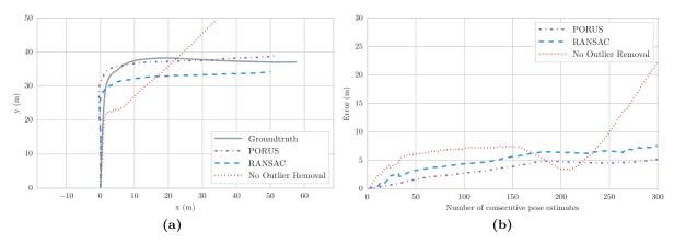
**Figure 7.13:** KITTI 2009\_09\_08\_drive\_0010 (a) Reconstructed trajectories. (b) Euclidean distance error of estimated trajectories as a function of the number of pose estimates.
