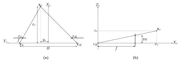
**Figure 2.5:** Geometry of rectified, stereo camera coordinate system. (a) Top down view of stereo pair geometry. (b) Side view of stereo pair geometry. Adapted from Brink [51, Figure 3.6].
