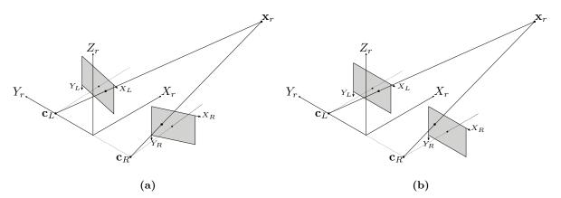
**Figure 2.4:** Image rectification of stereo camera pair. (a) An unrectified stereo camera pair. (b) The resulting camera system after image rectification has been performed, where the epipolar lines of both image planes are parallel to the baseline.
