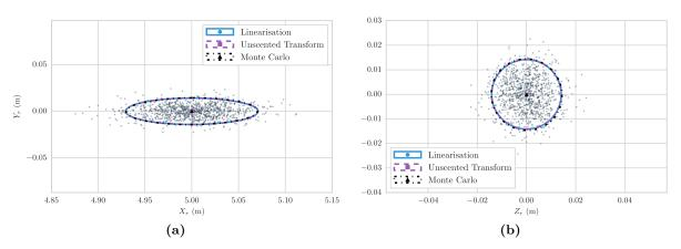
Figure 3.4:  $2\sigma$  contour plots and means of linearisation and unscented transform approximations for at a distance of 5.0 m from the stereo camera pair. (a)  $X_r - Y_r$  projection of 3D feature distribution. (b)  $Z_r - Y_r$  projection of 3D feature distribution.
