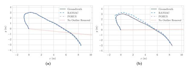
Figure 7.10: Synthetic visual odometry results. Example reconstructed robot trajectories after PORUS, RANSAC and no outlier removal are performed on a synthetic dataset. (a) No measurement noise and an inlier ratio of  $\epsilon = 0.8$ . (b) Measurement noise of  $\sigma = 0.5$  px and an inlier ratio of  $\epsilon = 0.8$ .
