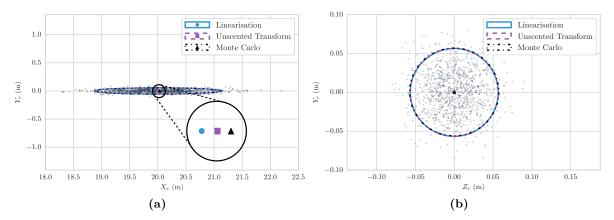
Figure 3.5:  $2\sigma$  contour plots and means of linearisation and unscented transform approximations for a distance of 20.0 m from the stereo camera pair. (a)  $X_r - Y_r$  projection of 3D feature distribution. (b)  $Z_r - Y_r$  projection of 3D feature distribution.
