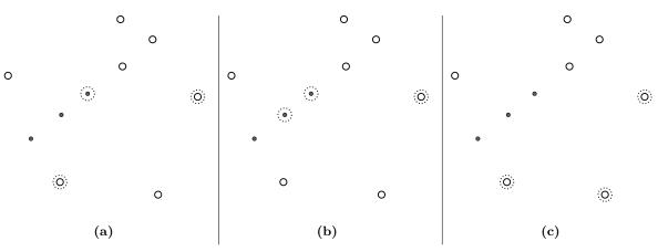
**Figure 6.4:** Different sampling strategies available after a set of inlier points has been identified. Sampled points are indicated by dashed circles. (a) A single inlier and two uncertain points are sampled. (b) Two inlier points and a single uncertain point are sampled. (c) Three uncertain points are sampled.
