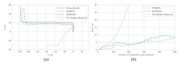
**Figure 7.14:** KITTI 2009\_09\_08\_drive\_0016 (a) Reconstructed trajectories. (b) Euclidean distance error of estimated trajectories as a function of the number of pose estimates.
