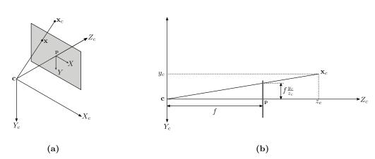
Figure 2.1: A basic pinhole camera model. (a) The camera centre, **c**, is defined at the origin of a camera coordinate system with an image plane (shaded) that meets the principal axis at the principal point, **p**. A 3D point,  $\mathbf{x}_c$ , is projected to a 2D image coordinate, **x**. (b)  $Y_c - Z_c$  plane view of pinhole camera model. Adapted from Hartley and Zisserman [62, Fig. 6.1].
