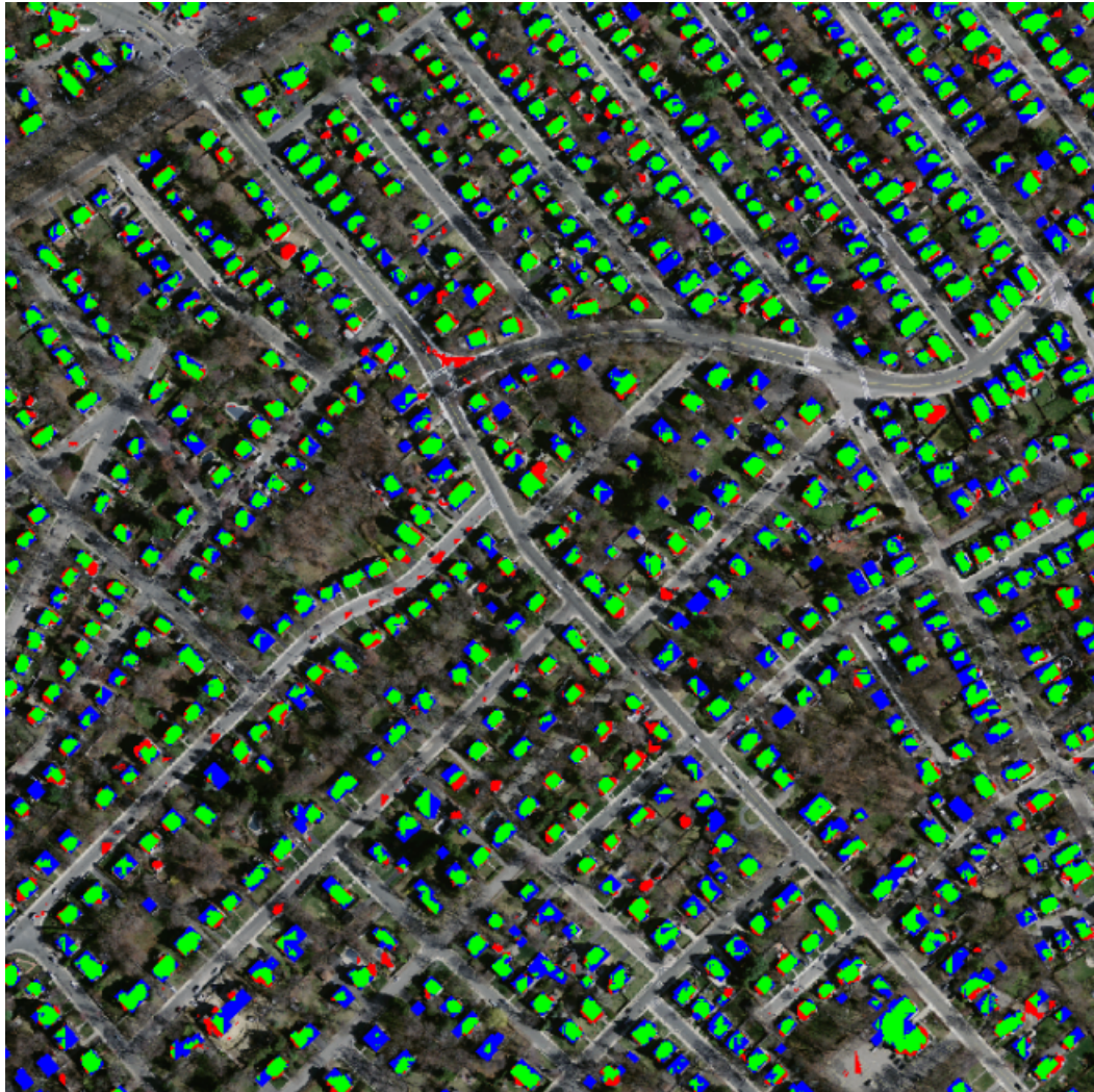
Figure 3.6: the image is the map predicted by our base model (without dropout, and post-processing) overlaid on the actual image. The green parts are true positives, the red parts are false positives, the blue parts are false negatives and the rest are true negatives.
