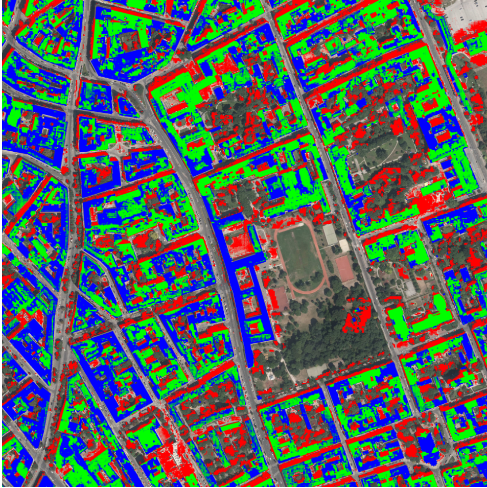
Figure 4.8: The predictions made by our MBD trained model (green parts in the image) are overlaid on one of the Inria dataset. The red parts are the false positives and the blue parts are the false negatives.
