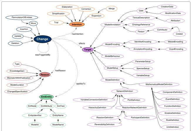
Fig. 2 Structure of the COMODI ontology. Differences between computational models can be annotated with the Change term. Using the properties appliesTo, hasIntention, hasReason, and affects, the differences can be linked to the terms of the four major branches of COMODI: XmlEntity, Intention, Reason and Target. All arrows between terms within these five branches indicate an is-a relation, unless labelled otherwise
