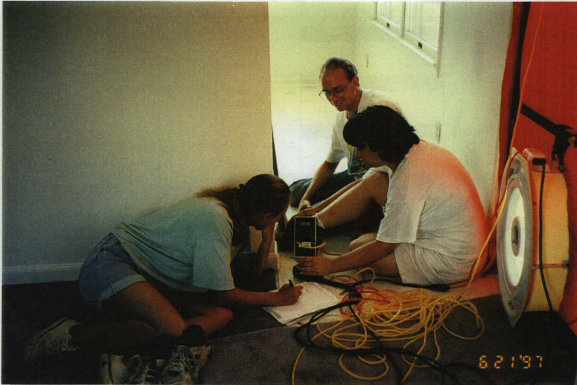
Figure 8-5, Air Tightness Testing
