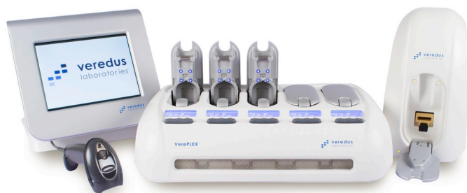
Fig. 13. The VerePLEX™ Biosystem consists of two main parts: (i) the temperature control system, which can process up to 5 cartridges independently and simultaneously, and supports multiplex PCR (middle in the above figure – W \times H \times D: 50.0 \times 14.5 \times 30.0 cm; weight: 10.0 kg); and (ii) the optical reader, which detects the microarray on the chip within seconds based on CCD imaging technology (right in the above figure – W \times H \times D: 18.0 \times 31.0 \times 18.0 cm; weight: 3.6 kg). A laptop/PC is also necessary for control and software handling. Image source: used from [118].
