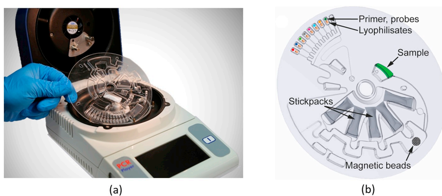
Fig. 24. (a) Image of the LabDisk and corresponding processing device (W × H × D: 17.5 × 30.0 × 28.0 cm; weight: 2.0 kg). (b) Schematic of a typical LabDisk design for sample-to-answer nucleic acid analysis. The figure indicates the pre-storage of all necessary reagents. Image sources: (a) Hahn-Schickard, Bernd Müller Fotografie; (b) Hahn-Schickard, F. Stumpf.
