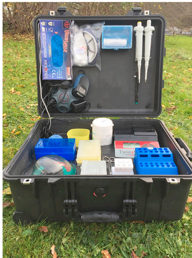
Fig. 28. Assembly of the Diagnostics-in-a-Suitcase (W × H × D: 56.0 × 26.5 × 45.5 cm; weight: 8.0 kg). A PVC layer is placed on top of the foam to fill the bottom of the suitcase. The equipment is fixed to the PVC layer using hot glue. The suitcase includes a tube scanner, the box for the disinfection wipes, the waste container, the vortex, the pipette tips, the minicentrifuge, and two boxes of refill pipette tips. Also, electricity wires are stowed underneath the foam layer. Image sources: reprinted from [186], Copyright © 2015, with permission from the open access article distributed by the journal under the Creative Commons Attribution License.
