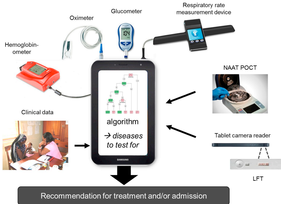
Fig. 30. Electronic decision making algorithm supported by a tablet connected to sensors, a NAAT POC test, and LFTs (through an LFT automated reader). Source: Valérie D’Acremont and Kristina Keitel.
