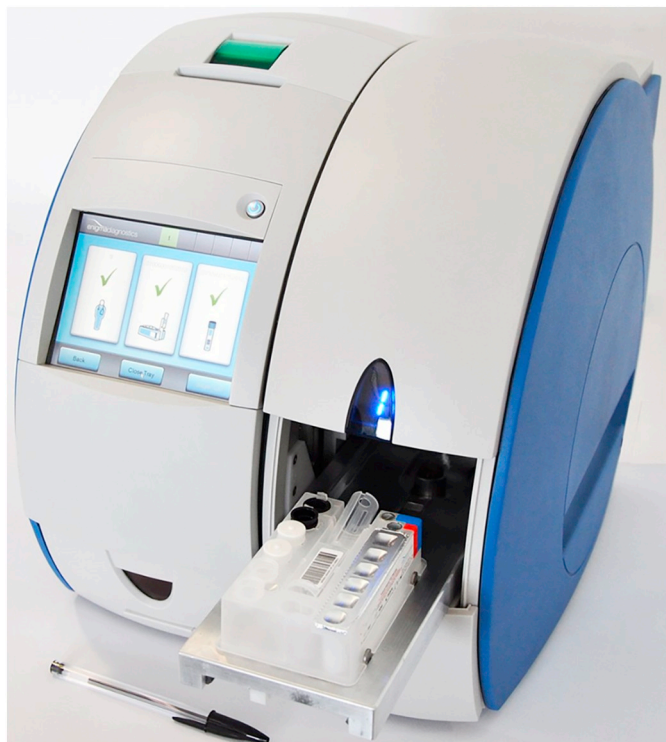
Fig. 9. Single-module configuration of the Enigma® ML system (W × H × D for a single module: 31.5 × 35.5 × 43.0 cm; weight: 19.4 kg) indicating how the cartridge is inserted. Image source: reprinted from [106], Copyright © 2016, with permission from the American Society for Microbiology.
