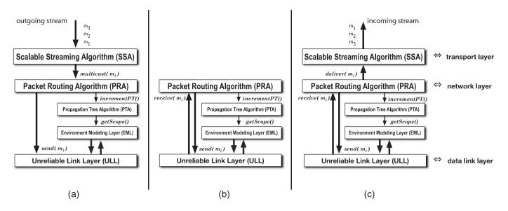
FIGURE 2. A layered architecture: (a) producer and router, (b) pure router and (c) consumer and router.
