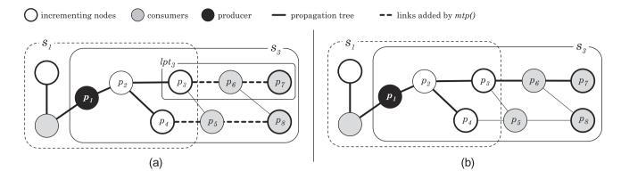
FIGURE 3. Propagation tree increment: (a) before the return statement and (b) returned propagation tree.
