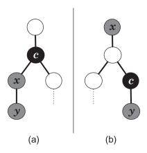
**FIGURE 10.** Two conflicting propagation trees received by c: (a) propagation tree  $T_1$  (received first) and (b) propagation tree  $T_2$  (received later).
