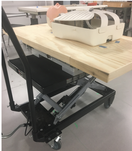
Figure 5: Manikin, force plate, and hydraulic cart set up for LH, KH, and WH. The hydraulic cart height was adjusted to the desired height, using a foot pedal, within the CPR position.
