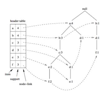
Figure 2.9: FP-tree with its header table
