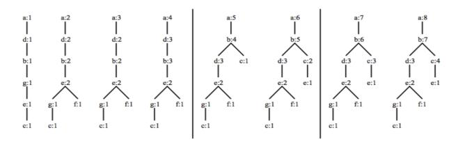
Figure 2.11: CATS tree in addition of each transaction of Table 2.6 (from left to right) [45]
