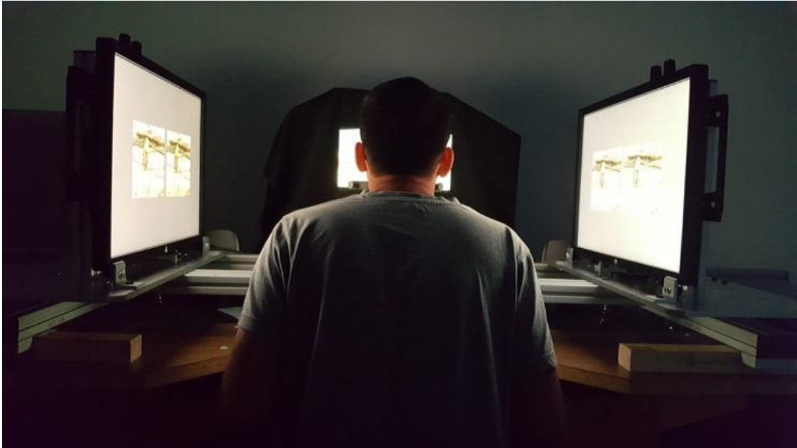
Figure 3.2: Set up of experiment showing a subject detecting the flickered image by using a gamepad. The head is placed in front of the mirrors using a chin rest at a viewing distance of 45cm from each eye to its corresponding monitor.
