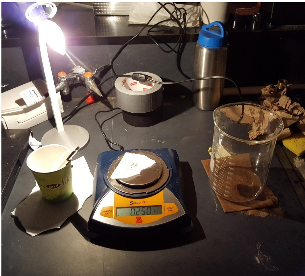
Figure 2.8 – SiO 2 particles measured on digital scale. The beaker at the right would be used to remove water from the aquarium, and the particles would be added to the beaker and stirred.
