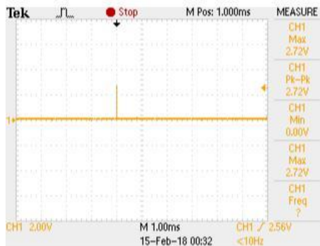
Figure 49: Low SD signal with noise at speed = 500 Hz
