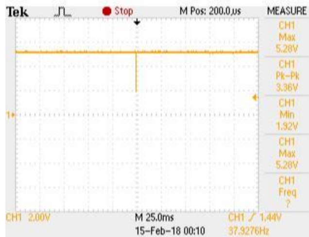
Figure 48: High SD signal with noise at speed = 500 Hz
