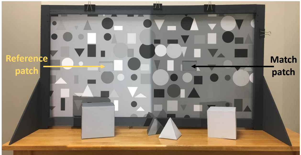
Figure 4.2 Photograph of the experimental apparatus. The left rectangle is the reference aperture and the right rectangle is the match aperture.
