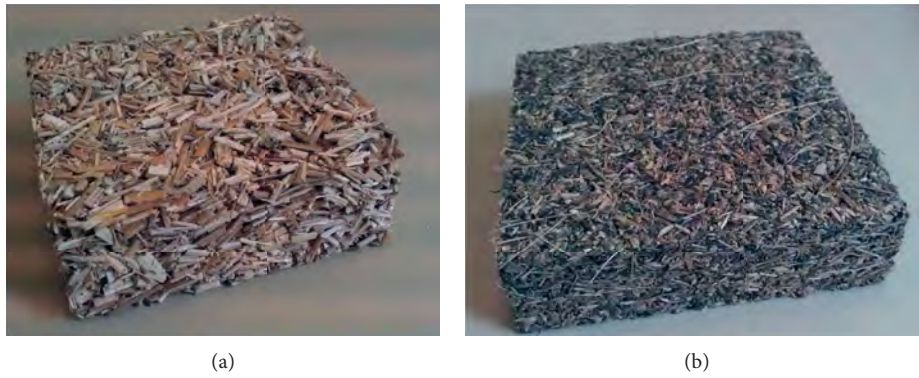
FIGURE 1: Composite materials. (a) Miscanthus fiber panel. (b) Sunflower stalk fiber panel.
