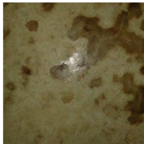
Fig. 11. Thermopressed sheet of cellulose-g-PDMDMA.
