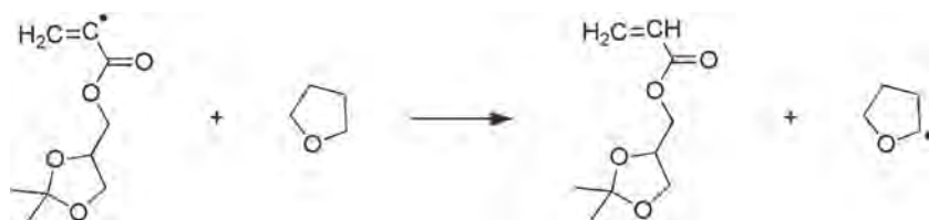
Scheme 3. Competitive reactions during the polymerization reaction in the presence of THF.
