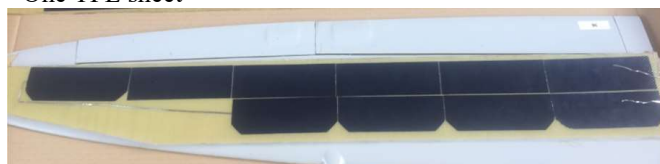
Fig. 12 Final encapsulation of PV cells
