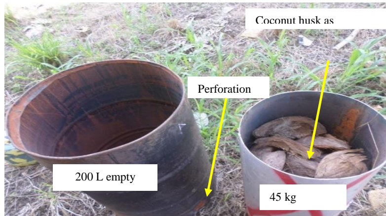
Figure 2. Pyrolysis oven consist of a 200 L drum and 45 kg cylinder for charring coconut husk.
