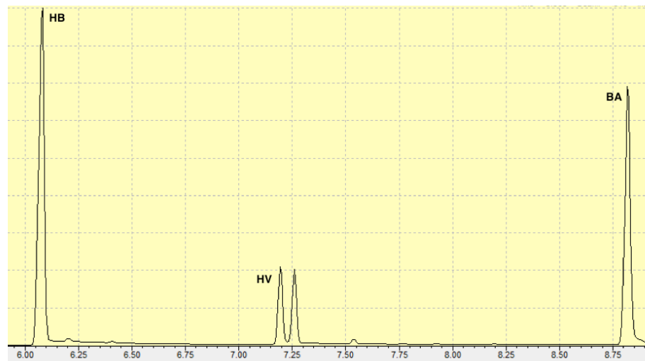
Figure 10: GC spectrum of the polymer isolated from the biomass, HB = hydroxybutyrate; HV = Hydroxyvalerate, BA = Benzoic acid internal standard.
