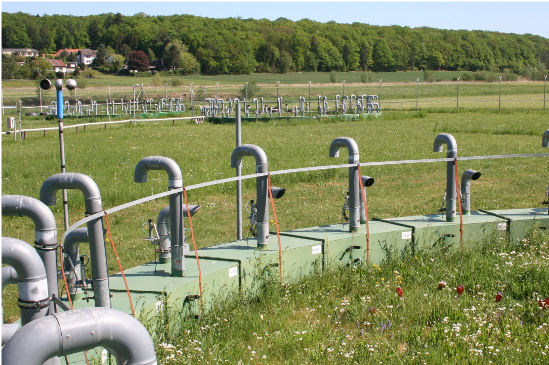
Figure 3.1: Experimental plots for the CO 2 enrichment at the Giessen FACE site.
