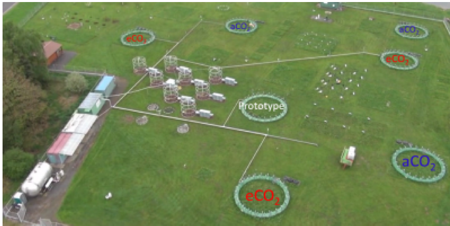
Figure 5.8: Aerial photo of the Gi-FACE field site. Locations of the rings with elevated \text{CO}_2 ( \text{eCO}_2 ) and ambient \text{CO}_2 ( \text{aCO}_2 ) are indicated. Inner diameter of the rings is 8m. We acknowledge the Hessian Agency for Nature Conservation, Environment and Geology (HLNUG) for providing this photo.
