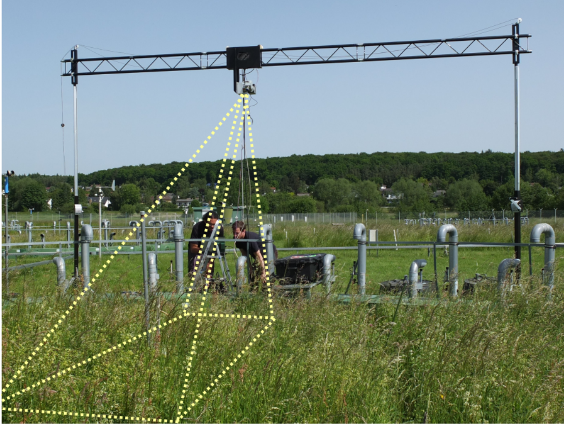
Figure 8.1: Hyperspectral measurement setup with the scanner mounted on a traverse system ( \sim 3 m height) above a \text{CO}_2 enrichment ring with releasing (lower) and absorbing (higher) vent pipes. The yellow dashed lines depict the approximate field of view for one image scan.
