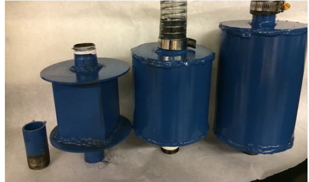
FIGURE 6. THE AIR CAPACITORS BUILT FOR THIS SETUP THAT ALLOWED FOR DIFFERENT INTAKE MANIFOLD VOLUMES
