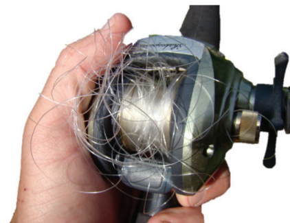
Figure 2 - A "bird's nest" resulting from poor cast control
