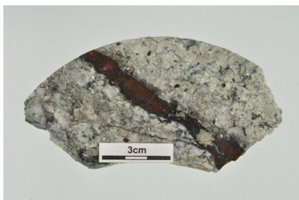
Fig. 2. Segment of Rookhope Borehole core, depth 1647 feet (502 m), consisting of Weardale Granite cut by bitumen-bearing quartz vein (dark) mineralized by pyrite. The quartz-bitumen vein is cut by a thin fluorite-bearing vein.
