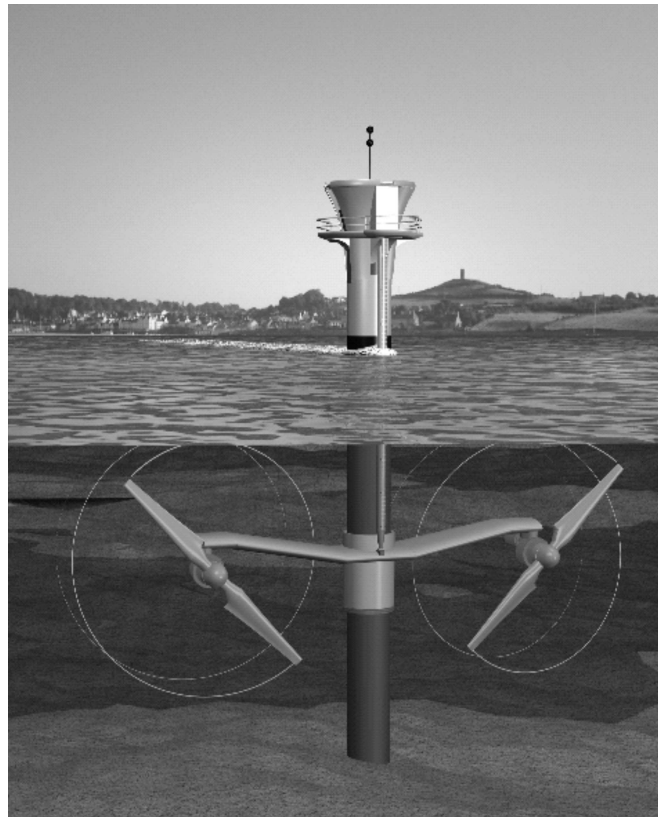
Figure 2. Artists impression of the Seagen Marine Current Turbine.
