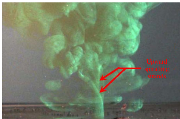
FIGURE 7. (Colour online) Fluorescein visualization of the stem of a jet revealing the two cyclonically upward-spiralling helical strands for Re_0 = 2300 at \Omega = 0.21 \text{ rad s}^{-1} . A supplementary movie is available at https://doi.org/10.1017/jfm.2019.186 .
