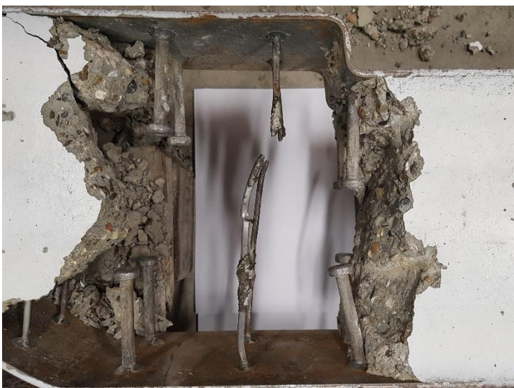
Figure 22: Steel plate local buckling of SCB1
