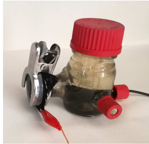
Fig. 2. Picture of the Single Chamber Microbial Fuel Cell: a Pyrex® bottle of 0.125 L volume equipped with the air-breathing cathode on the opening on the left side, the anode connected through the small opening on the right side and the big opening on the top for positioning the sample electrode.
