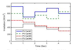
Figure 10. Step change of solar irradiation with PSC.
