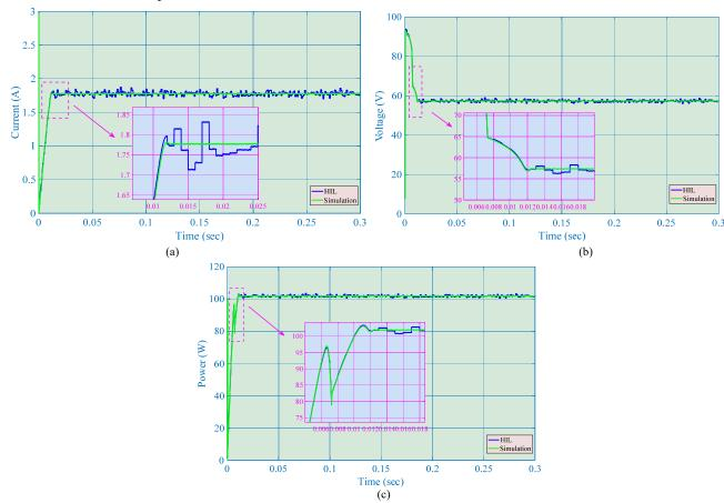
Figure 19. The simulation results and HIL test results obtained under the start-up test. (a) Current, (b) Voltage, (c) Power, and (d) Energy.
