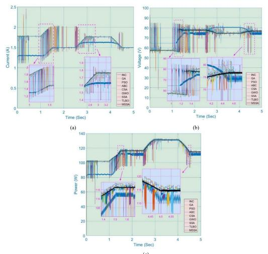
Figure 13. PV system responses of seven methods obtained on the gradual change in both solar irradiation and temperature. (a) Current, (b) Voltage, and Power.
