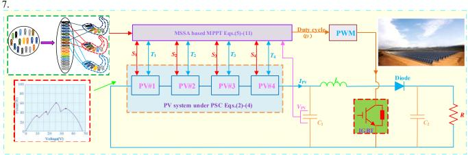
Figure 6. Overall structure of MSSA based MPPT of PV system under PSC.
