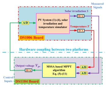
Figure 17. The configuration of HIL experiment.
