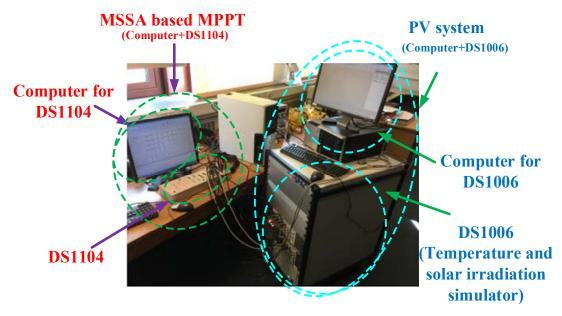
Figure 18. The hardware platform of HIL experiment.
